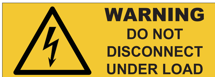
Figure B.13 — Typical battery system isolator sign
