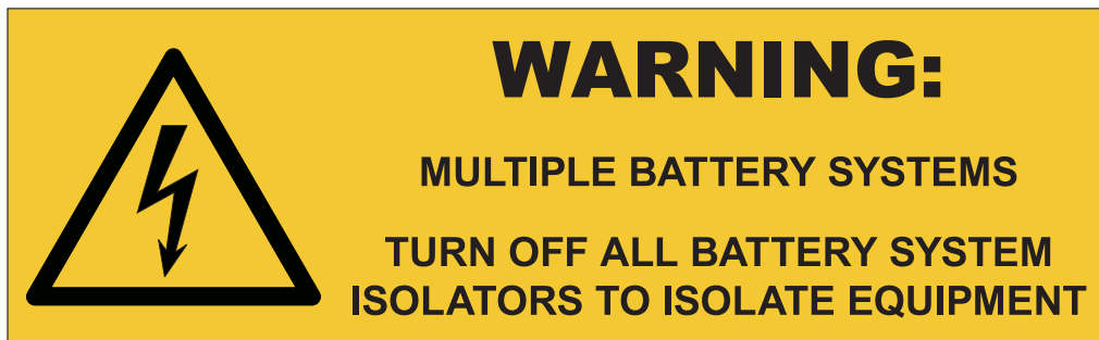
Figure B.12 — Typical battery system isolator sign
